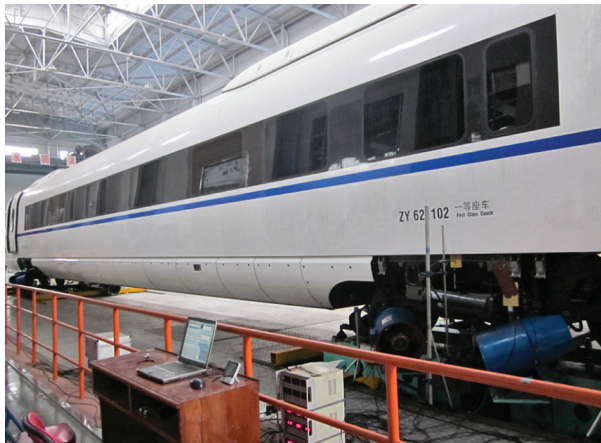
Fig. 1. Test scene of the rolling and vibrating test-bed
